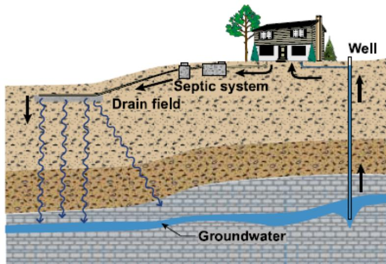
**Figure 6. On-Lot Disposal System and Groundwater Flow**
