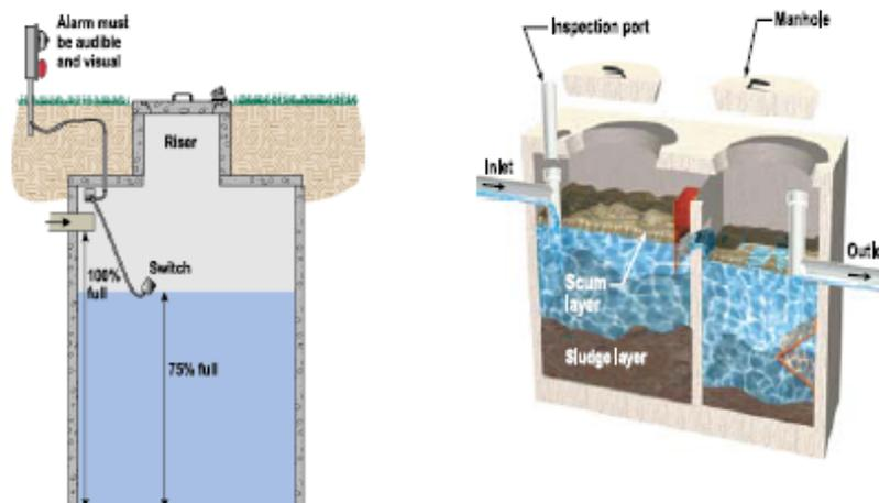
**Figure 3. Comparison of Holding vs. Septic Tank**
