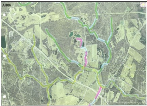
Above left: Riparian forest buffer inventory desktop survey for stream segments. Green highlighted stream segments were classified as Class 1 RFBs, yellow Class 2, and red Class 3. Above right: Total number of acres for each buffer class identified in York County's Riparian Forest Buffer Inventory.
