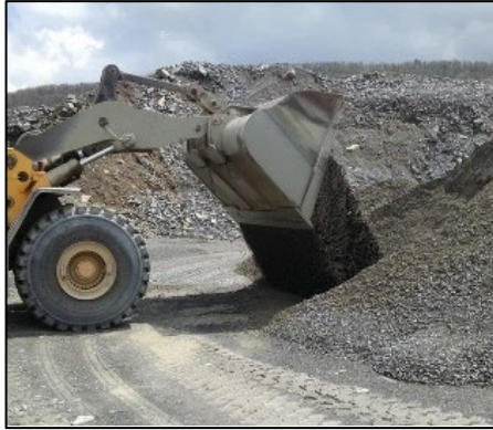
Figure 2. Laying out the sampling pile
